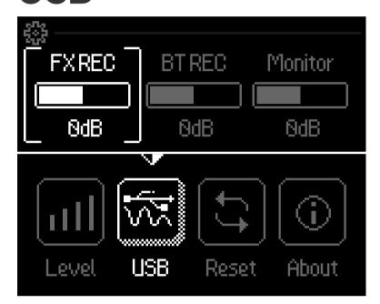
FX REC (Effect recording volume): Adjust the volume of the effect audio recording, ranging from-20dB to 20dB.
